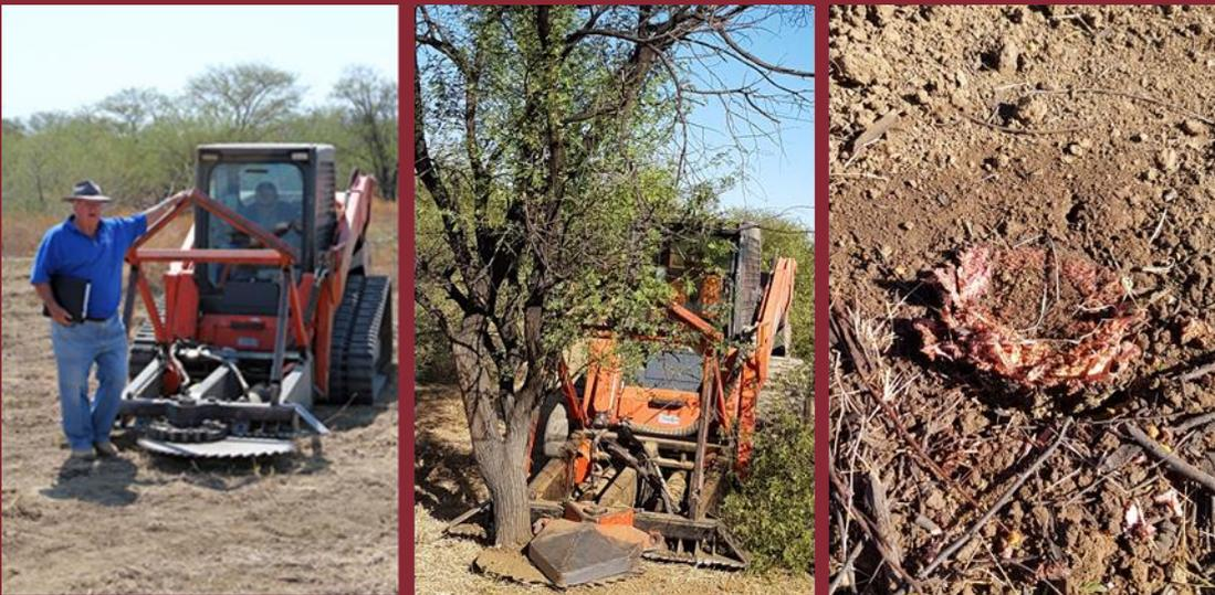
Figure 1. Marshall Tree Saw showing device mounted to a bobcat (left) treating prickly acacia (middle) and the sprayed cut surface of the stem (right).
